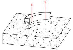
2 Put the housing in the hole and fix it with screws
